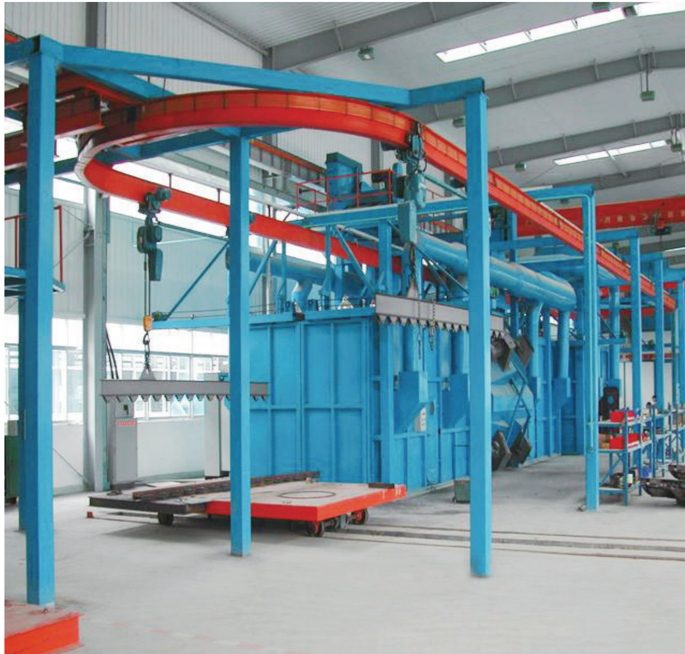
QT37系列环轨通过式抛丸清理机 QT37 Series Circular Track Through Type Shot Blasting Machine
